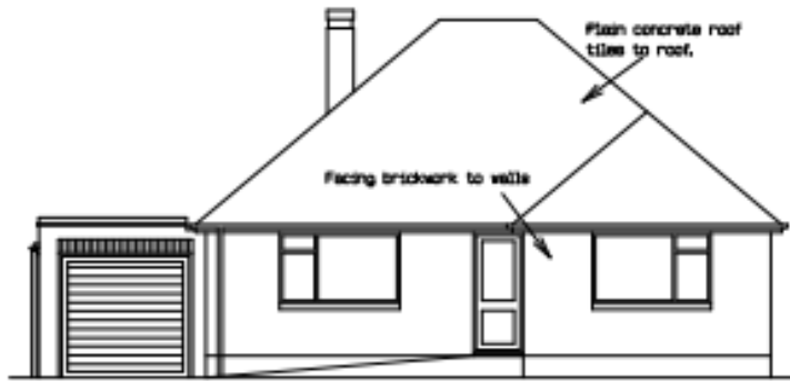
EXISTING FRONT ELEVATION
